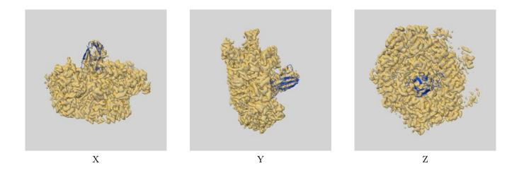
The images above show the 3D surface view of the map at the recommended contour level 0.01 at 50% transparency in yellow overlaid with a ribbon representation of the model coloured in blue. These images allow for the visual assessment of the quality of fit between the atomic model and the map.
