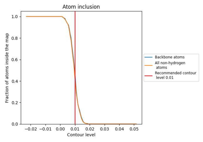
At the recommended contour level, 47% of all backbone atoms, 42% of all non-hydrogen atoms, are inside the map.
