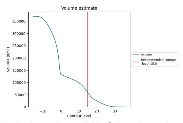
The volume at the recommended contour level is  $58596 \text{ nm}^3$ ; this corresponds to an approximate mass of 52932 kDa.
