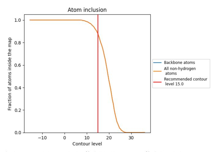
At the recommended contour level, 88% of all backbone atoms, 88% of all non-hydrogen atoms, are inside the map.
